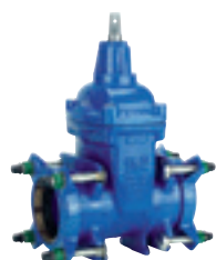
Series 01/70 Supa Plus™ gate valve Tensile for PE and uPVC pipes Ductile iron DN 40-300 PN 16
